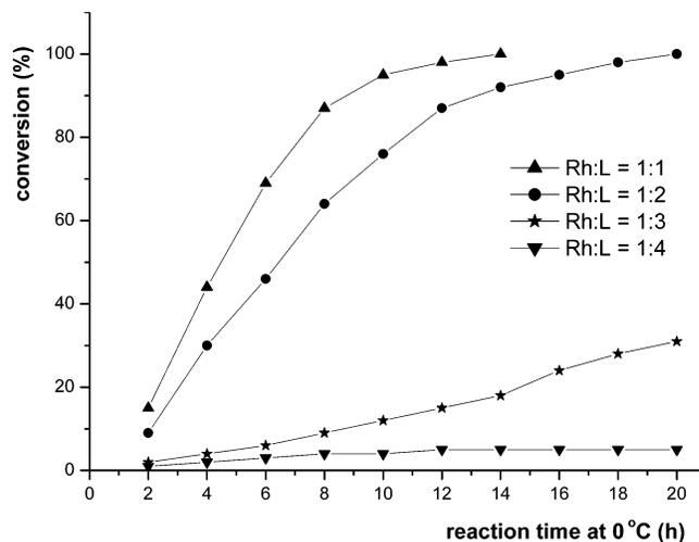
**FIGURE 8.** Dependency of conversion vs time at 0 °C.
