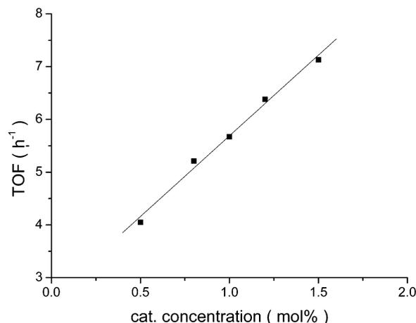
**FIGURE 4.** Dependency of TOF versus catalyst concentration ( $T = 25\text{ }^{\circ}\text{C}$ ,  $P_{\text{H}_2} = 1\text{ atm}$ ,  $[\text{sub}]_0 = 0.1\text{ M}$ ,  $[\text{Rh}] = 0.5\text{--}1.5\text{ mM}$ ).
