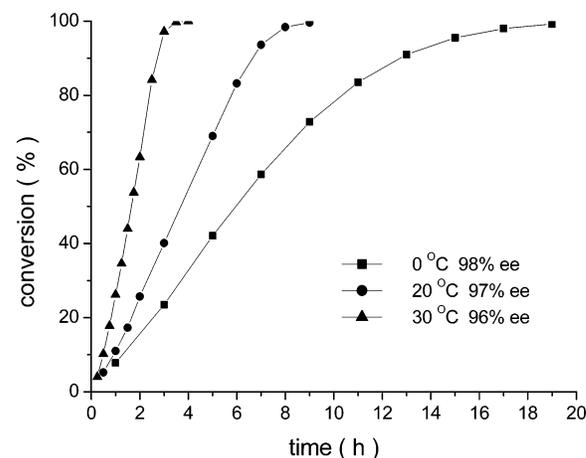
**FIGURE 6.** Dependency of reaction rate versus temperature ( $T = 0\text{--}30\text{ }^{\circ}\text{C}$ ,  $P_{\text{H}_2} = 1\text{ atm}$ ,  $[\text{sub}]_0 = 0.1\text{ M}$ ,  $[\text{Rh}] = 1.0\text{ mM}$ ).
