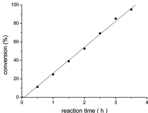
**FIGURE 3.** Dependency of conversion versus reaction time ( $T = 25\text{ }^{\circ}\text{C}$ ,  $P_{\text{H}_2} = 1\text{ atm}$ ,  $[\text{sub}]_0 = 0.1\text{ M}$ ,  $[\text{Rh}] = 1.0\text{ mM}$ ).
