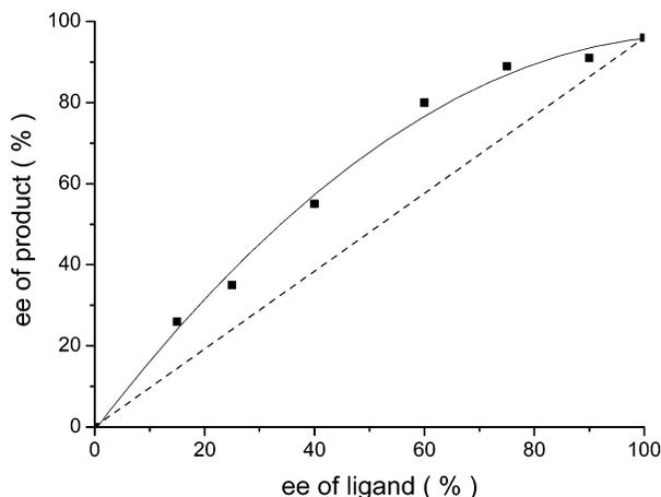
**FIGURE 7.** NLE in Rh/SIPHOS-catalyzed hydrogenation ( $T = 25\text{ }^{\circ}\text{C}$ ,  $P_{\text{H}_2} = 1\text{ atm}$ ,  $[\text{sub}] = 0.1\text{ M}$ ,  $[\text{Rh}] = 1.0\text{ mM}$ ,  $\text{Rh}/\mathbf{5a} = 1:2.1$ ).
